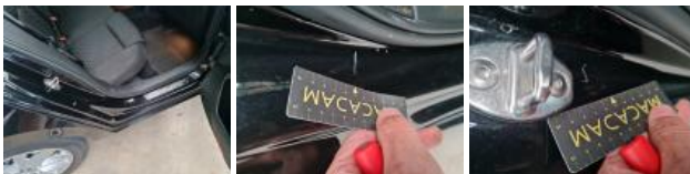
Outside rear-view mirror housing R, Scratch(es), Repair and paint (complete)
