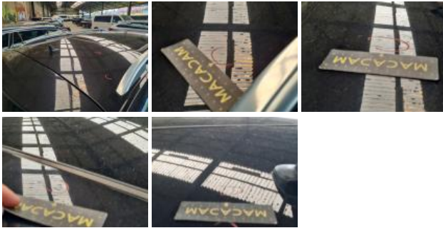
Roof, Hail damage, Paintless dent repair (hail)
