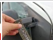
Side panel moulding R, Broken, Replace
