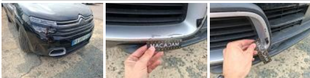
Bumper moulding F, Deformed / Strained, Replace
