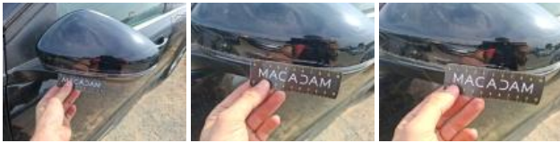
Side repeater L, Scratch(es), Replace
