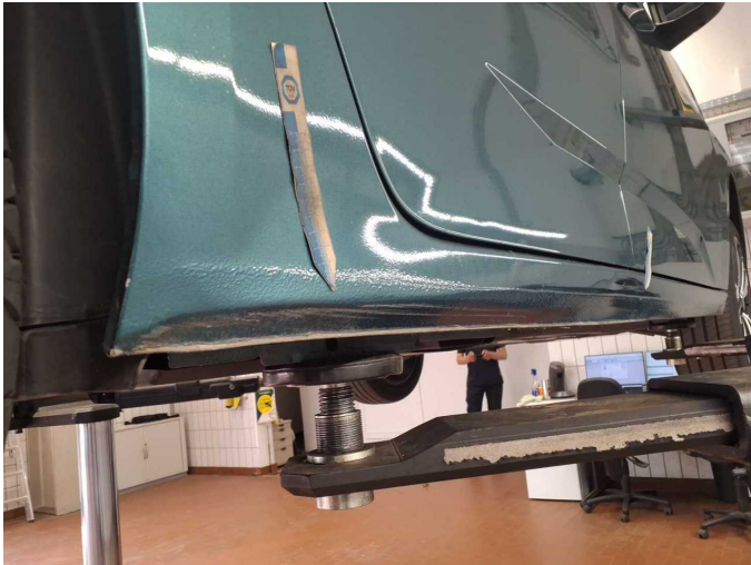
Damage 11: Sill - right side: Sill (+ Unterbodenschutz anbringen) - Deformed - Repair and paint
