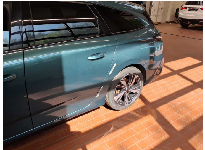
Damage 3: Side panel - rear left side: Elbow - dent(s) - Smooth repair work
