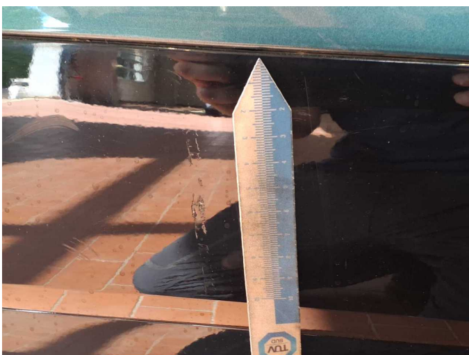
Damage 12: Rear bumper: Spoiler - Scratch(es) - Paint
