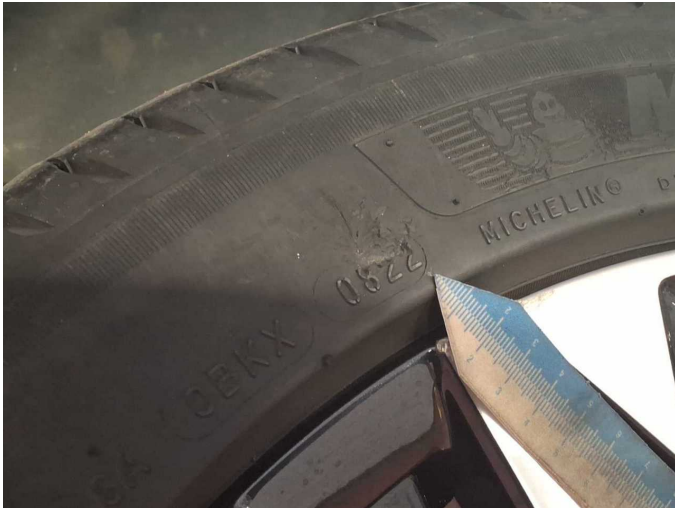
Damage 6: Wheel / tyres: Tyre - rear right side (nicht fahrbereit) - Broken / torn - Replace
