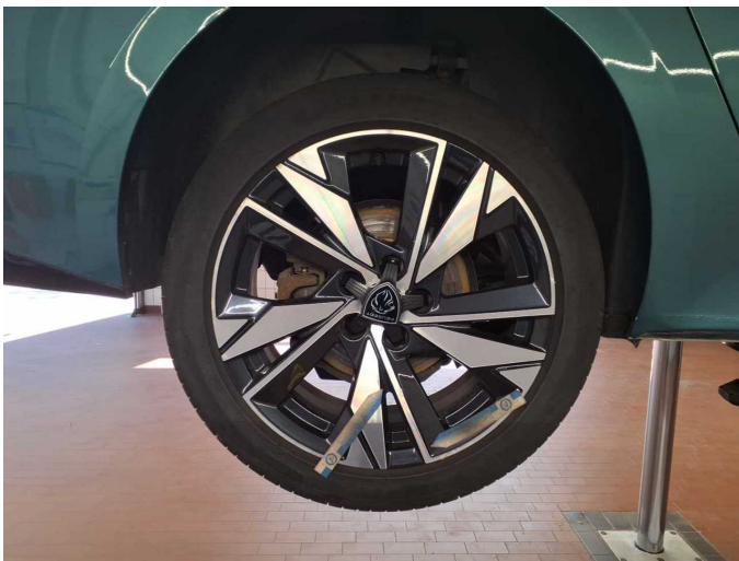
Damage 9: Wheel / tyres: Alloy rim - rear right side - Scratched - Replace
