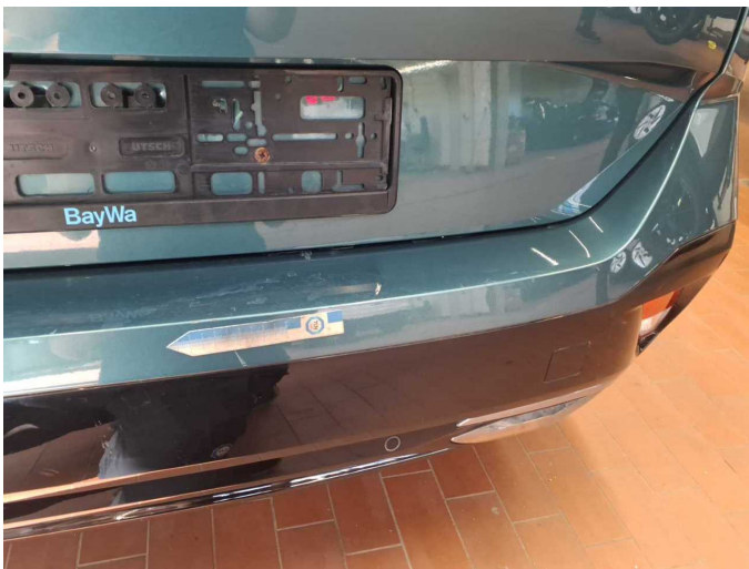
Damage 13: Rear bumper: Rear bumper - Dent / paintcoat damage - Repair and paint
