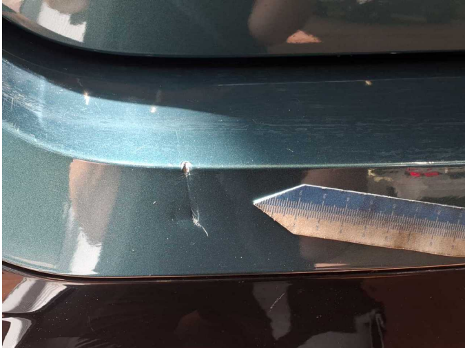
Damage 13: Rear bumper: Rear bumper - Dent / paintcoat damage - Repair and paint
