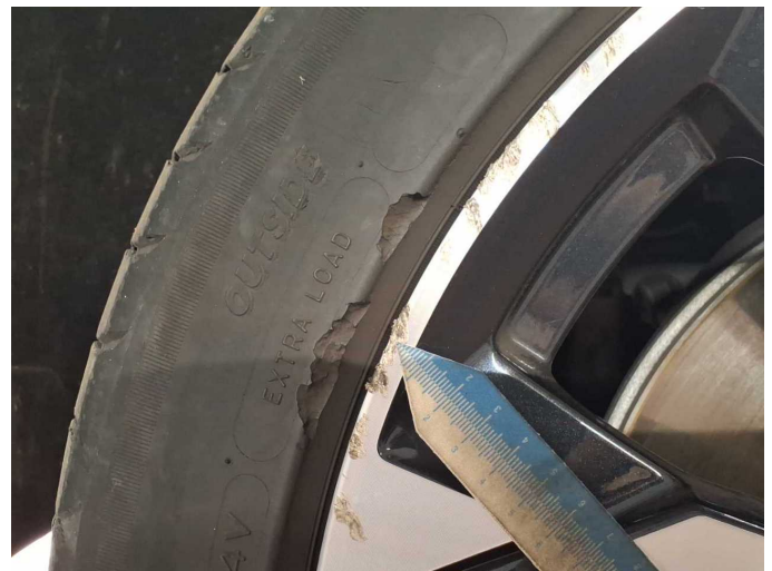
Damage 7: Wheel / tyres: Tyre - front right side (nicht fahrbereit) - Broken / torn - Replace
