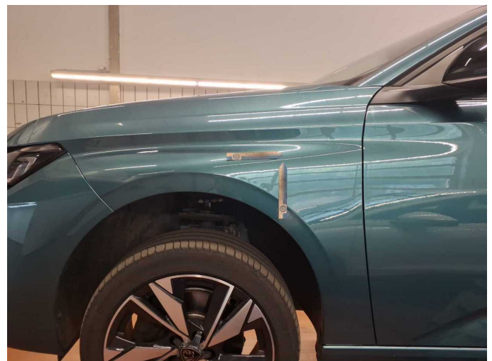
Damage 8: Mudguard - left side: Mudguard - left side - dent(s) - Smooth repair work
