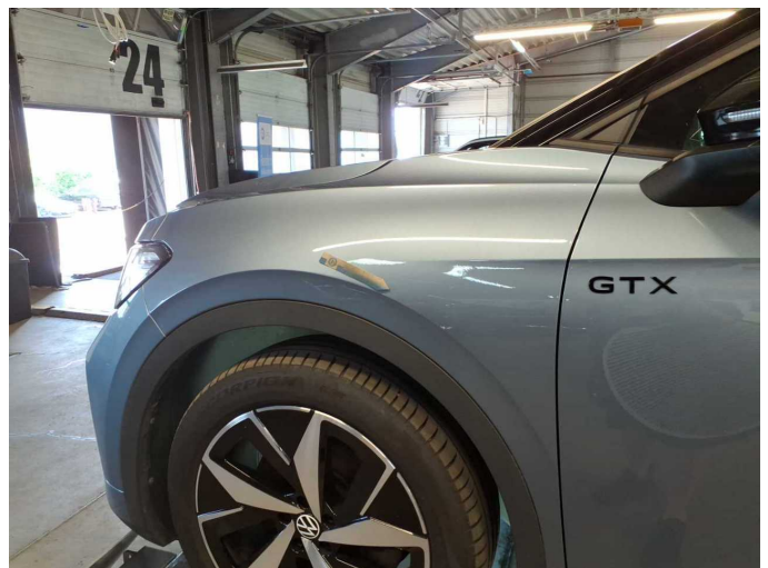
Wear and tear 2: Mudguard - left side: Mudguard - left side - Dent / paintcoat damage - No deduction
