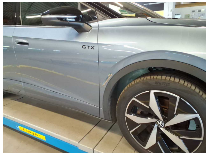
Damage 5: Mudguard - right side: Mudguard - right side - Dent / paintcoat damage - Smart repair
