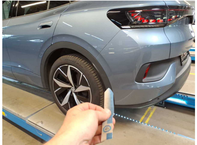
Damage 7: Side panel - rear left side: Wheel well extension - Scratch(es) - Replace
