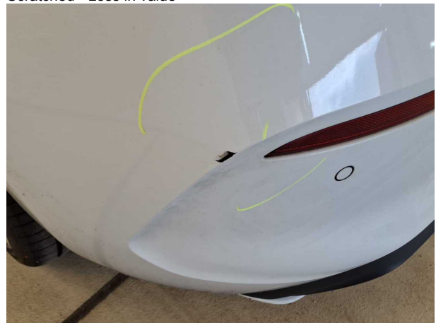
Damage #7: Rear bumper: Rear bumper - Scratched - Repair and paint
