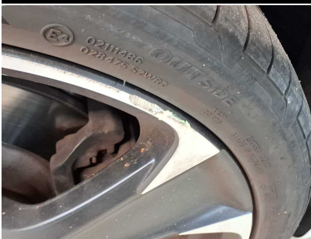
Damage #5: Wheel / tyres: Alloy rim - front right side - Scratched - Loss in value
