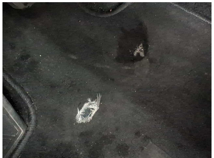
Damage 1: Trim / covers: Floor mats - Holes - Replace
