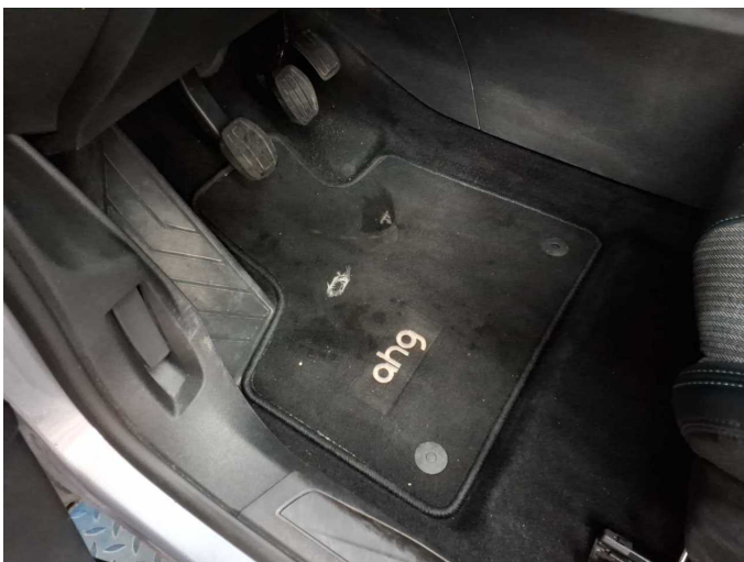
Damage 1: Trim / covers: Floor mats - Holes - Replace
