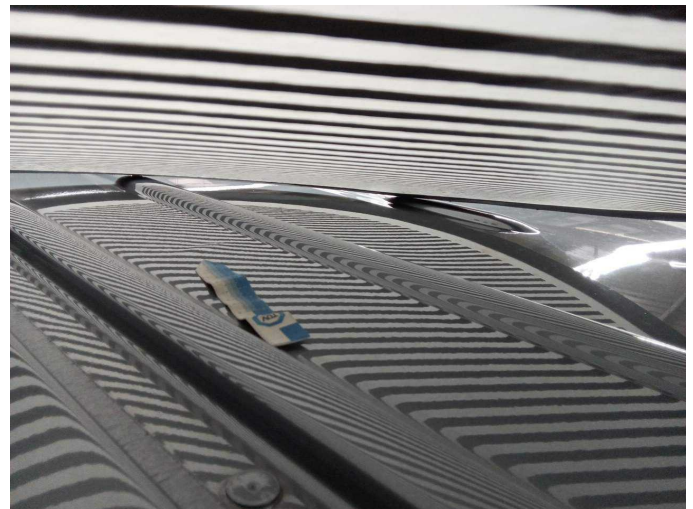
Damage 5: Roof: Roof - dent(s) - Smooth repair work
