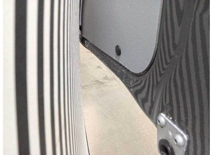
Damage 8: Boot lid / rear door: Rear door - right side (innem) - Dent / paintcoat damage - Smart repair
