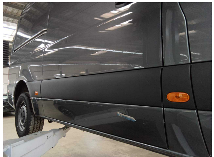
Damage 10: Sliding door, right: Sliding door (Unterhalb) - Scratch(es) - Smart repair
