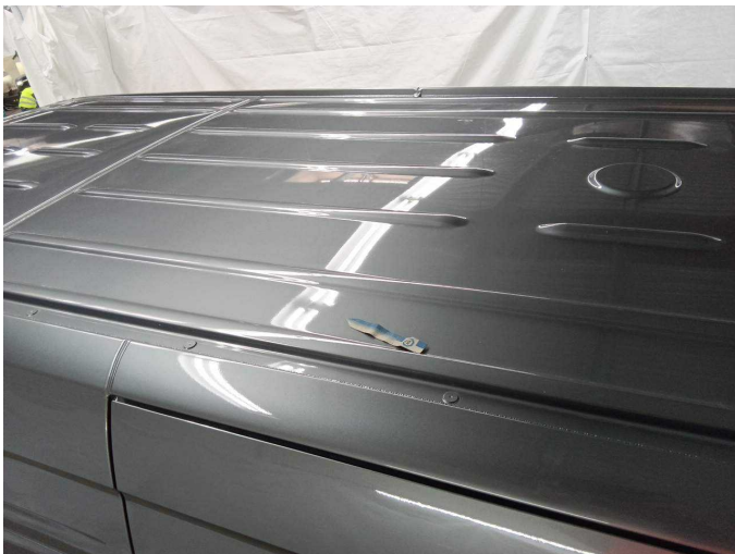
Damage 5: Roof: Roof - dent(s) - Smooth repair work
