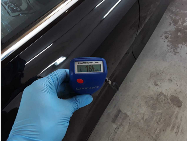
Repainting 1: Bonnet, Door - rear right side
