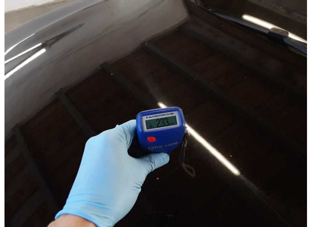
Repainting 1: Bonnet, Door - rear right side
