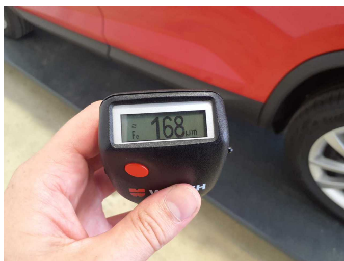
Repainting 4: Door - rear left side
