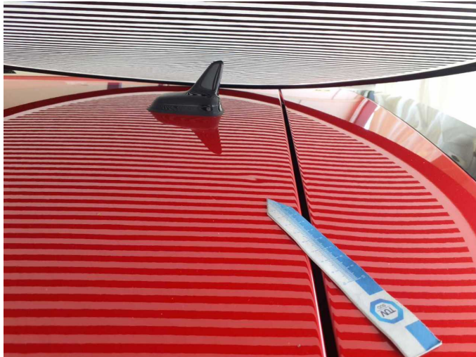
Damage 3: Roof: Roof - dent(s) - Smooth repair work
