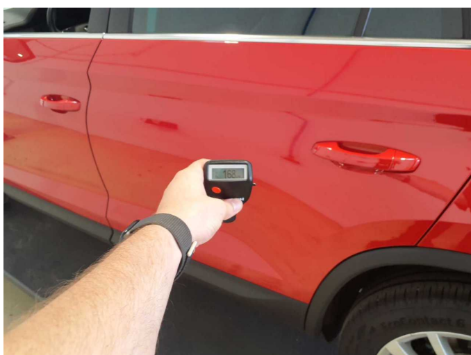
Repainting 4: Door - rear left side
