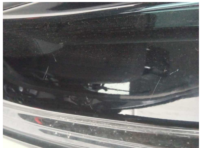
Damage 6: Side panel - rear left side: Sill - Dent / paintcoat damage - Repair and paint
