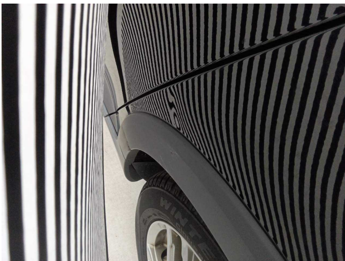
Damage 2: Side panel - rear left side: Mudguard - rear left side - dent(s) - Smooth repair work
