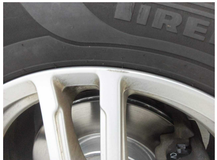
Wear and tear 8: Wheel / tyres: Alloy rim - front right side - Scratch(es) - No deduction
