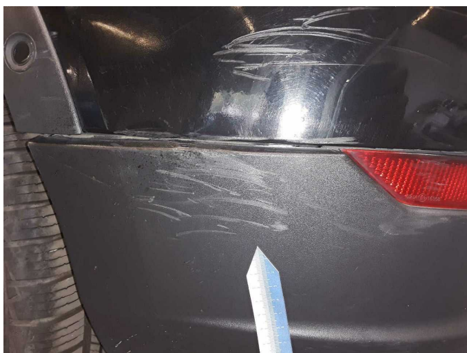
Damage 17: Rear bumper: Spoiler - Scratched - Replace
