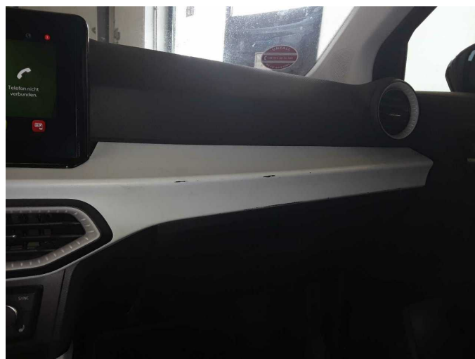
Damage 11: Instrument panel: Dashboard - right side - Scratch(es) - Loss in value
