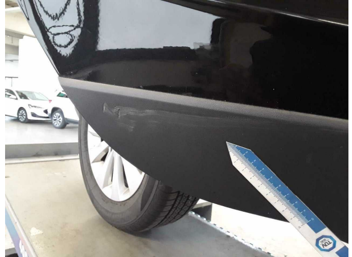
Damage 3: Trim / covers: Door trim - rear right side - Scratched - Replace
