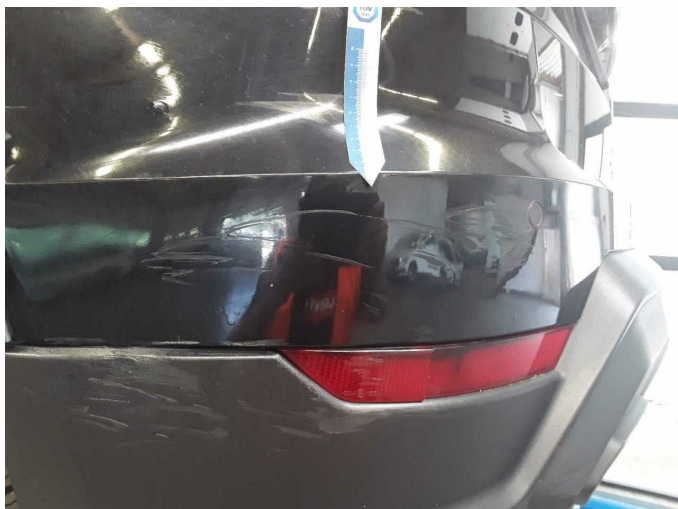
Damage 18: Rear bumper: Rear bumper - Scratched - Paint
