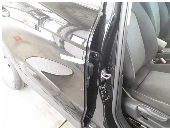
Damage 20: Door - rear right side: Door - Dent / paintcoat damage - Repair and paint
