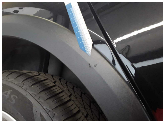
Damage 5: Side panel - rear right side: Wheel arch - Scratched - Replace
