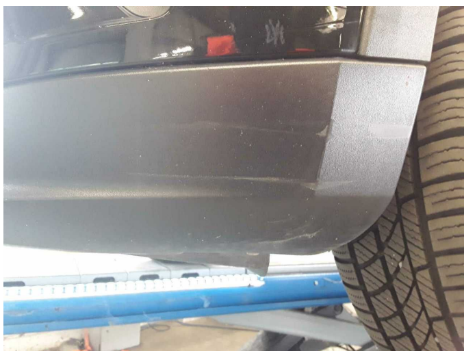
Damage 14: Body: Underbody panelling - Scratched - Replace
