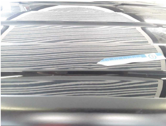
Damage 6: Roof: Roof - dent(s) - Smooth repair work
