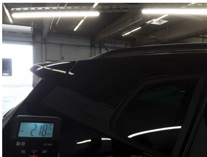
Roof rail - right side: 218 µm
