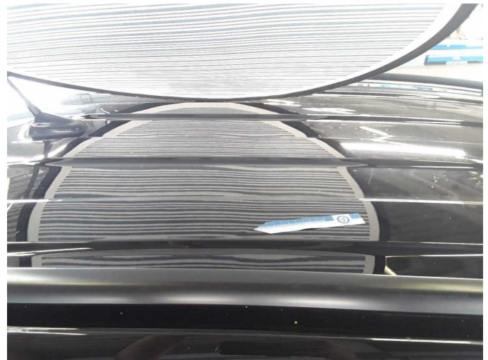
Damage 6: Roof: Roof - dent(s) - Smooth repair work
