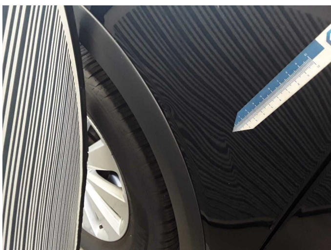
Damage 23: Mudguard - left side: Mudguard - left side - Deformed - Repair and paint
