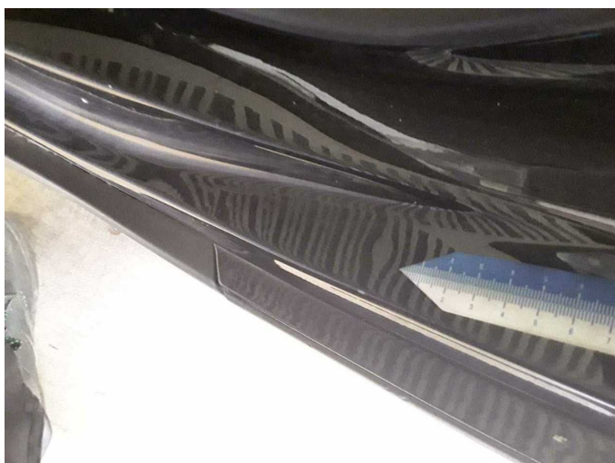
Damage 10: Side panel - rear left side: Elbow (Einstieg hinten) - Scratched - Smart repair
