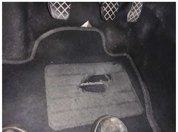
Damage 1: Trim / covers: Floor mats - Damaged - Replace
