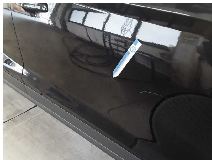
Damage 22: Door - front right side: Door - Scratch(es) - Paint
