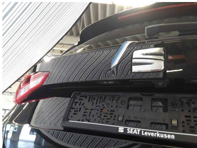
Damage 15: Boot lid / rear door: Boot lid - Dent / paintcoat damage - Smart repair
