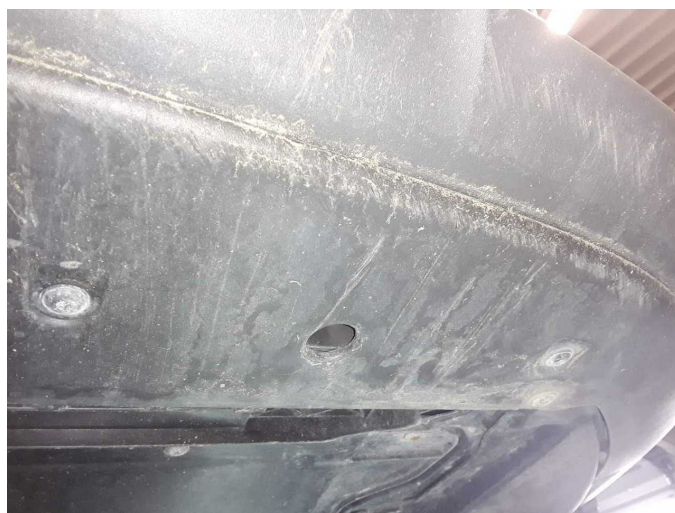
Damage 14: Body: Underbody panelling - Scratched - Replace
