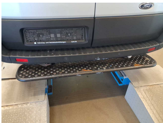
Damage 4: Rear of vehicle: Foot plate - Paint defect - Loss in value
