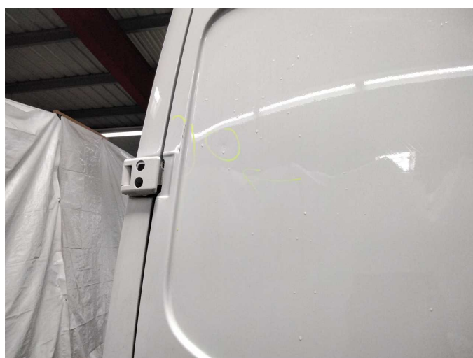
Damage 2: Boot lid / rear door: Rear door - left side - Dent / paintcoat damage - Smart repair
