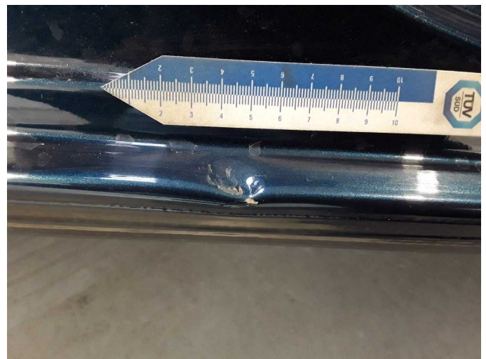
Damage 5: Sill - right side: Sill - Dent / paintcoat damage - Repair and paint
