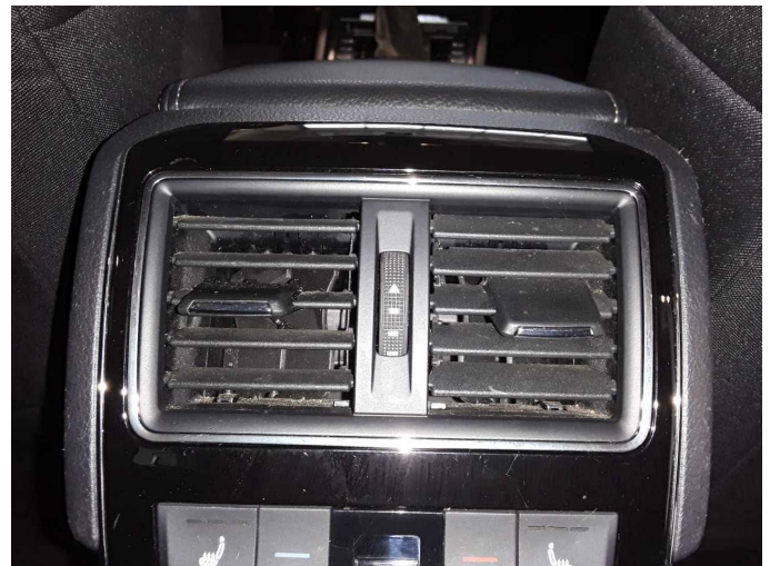
Damage 2: Instrument panel: Air nozzle - centre - Broken / torn - Replace
