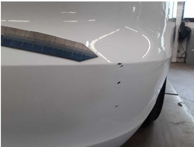
Damage 6: Rear bumper: Rear bumper - Scratch(es) - Paint
