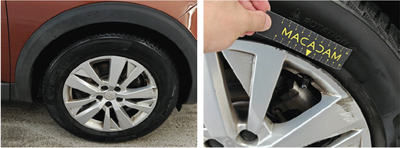
Alloy rim FR Scratch(es) Repair and paint (complete) Right
