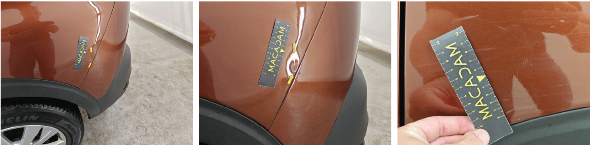
Wing RR Dent(s) and scratch(es) Repair and paint (complete) Right
