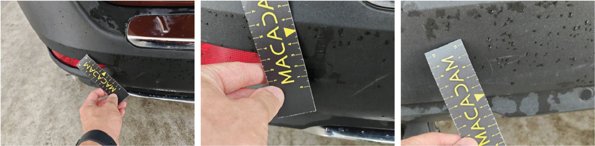
Door FL Dent(s) and scratch(es) Repair and paint (complete) Left
