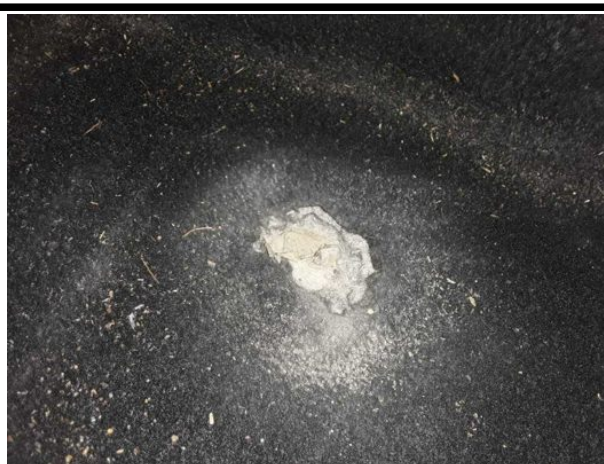
Damage #8: Trim / covers: Carpet - front left side - Holes - Replace
