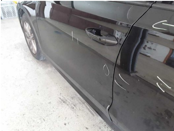
Damage #18: Door - front left side: Door - Dent / paintcoat damage - Repair and paint
