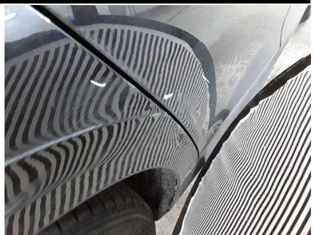
Damage #20: Side panel - rear right side: Side panel - Dent / paintcoat damage - Replace
