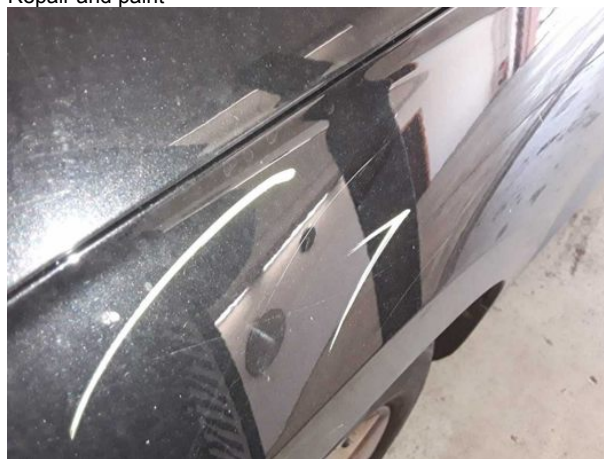
Damage #11: Mudguard - left side: Mudguard - left side - Scratched - Repair and paint
