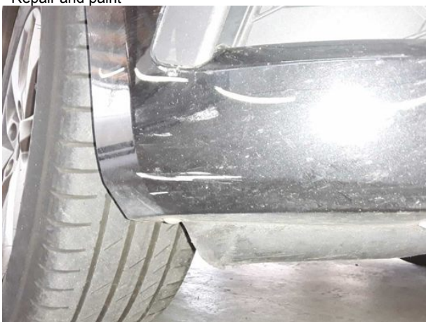
Damage #15: Front bumper: Front bumper - Scratched - Repair and paint
