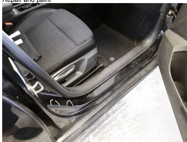
Damage #10: Sill - right side: Sill - Dent / paintcoat damage - Repair and paint
