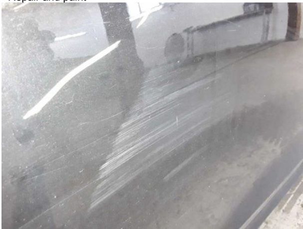
Damage #14: Door - rear right side: Door - Dent / paintcoat dama... - Repair and paint
