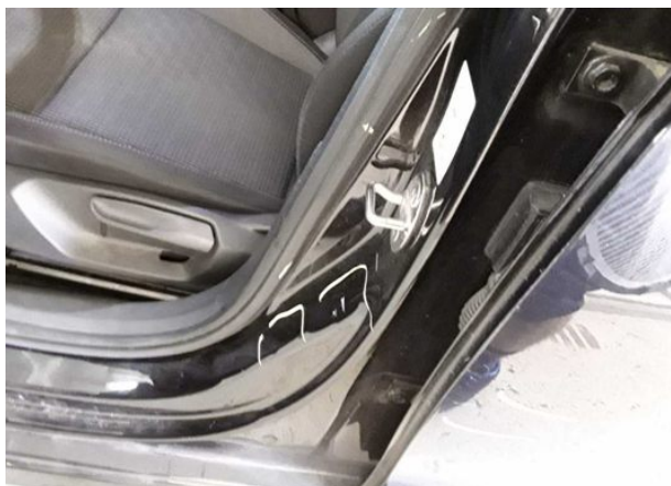
Damage #9: Sill - left side: Sill - Dent / paintcoat damage - Repair and paint
