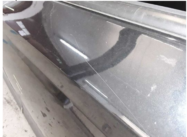
Damage #13: Door - rear left side: Door - Scratched - Repair and paint
