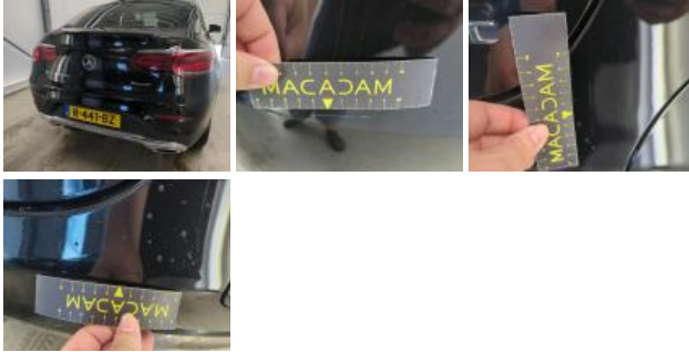
Bumper R, Scratch(es), Repair and paint (complete)
