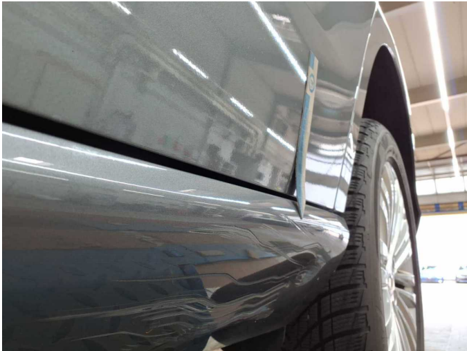
Damage 5: Sill - left side: Trim - Dent / paintcoat damage - Replace
