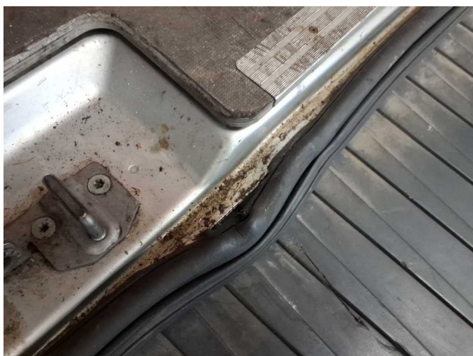
Damage 2: Boot lid / rear door: Seal - Malposition - Repair
