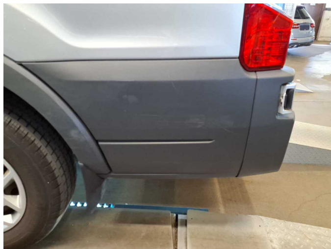
Damage 4: Side panel - rear left side: Side panel (Zierleiste) - Scratch(es) - Loss in value
