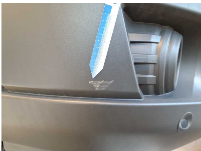
Damage 5: Front bumper: Front bumper (unpainted) - Scratch(es) - Smart repair
