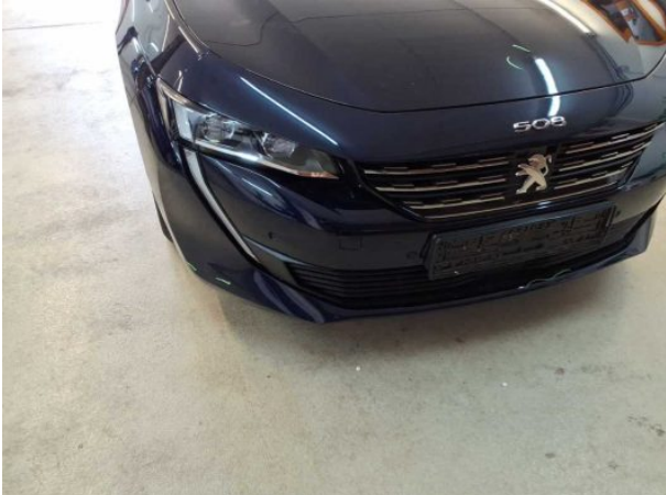
Damage #13: Front bumper: Front bumper - Scratched - Smart repair
