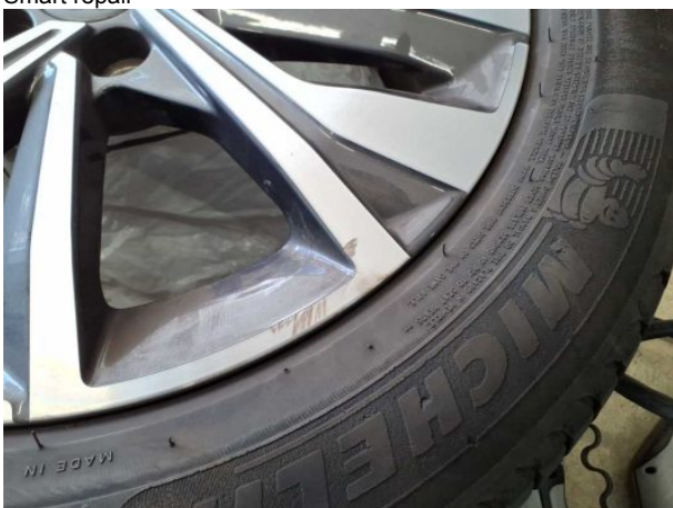
Damage #11: 2nd wheel set: 2 alloy rims - Scratched - Loss in value
