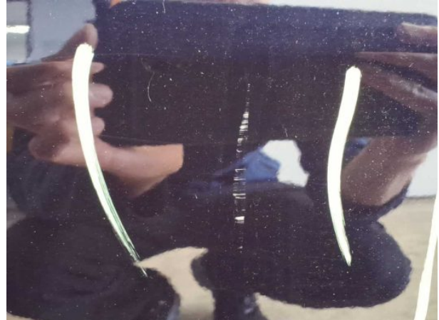
Damage #4: Door - front left side: Door - Scratch(es) - Cover / polish
