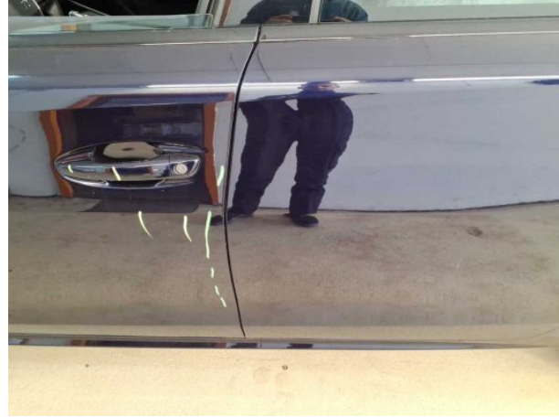
Damage #9: Door - rear left side: Door - Dent / paintcoat damage - Smart repair
