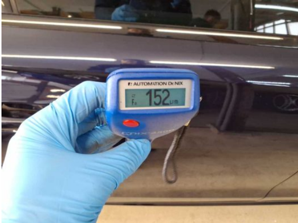
Repainting 1: Mudguard - right side, Side panel - rear right side, Door - rear right side
