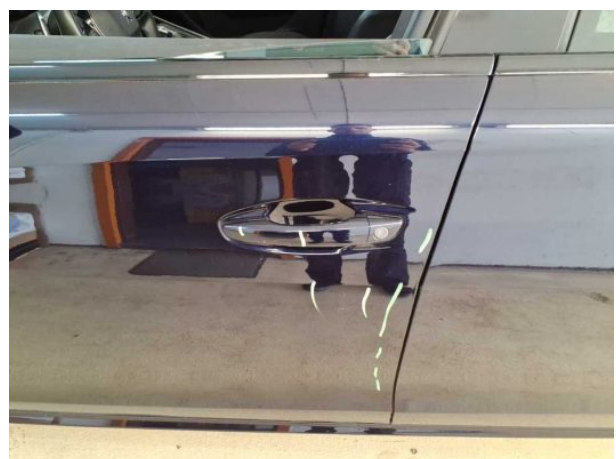
Damage #8: Door - front left side: Door handle - outside - Scratched - Smart repair
