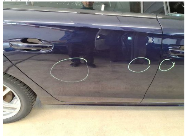
Damage #15: Door - rear right side: Door - Scratched - Repair and paint
