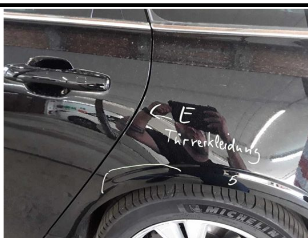
Damage #4: Side panel - rear left side: Side panel - Scratched - Smart repair
