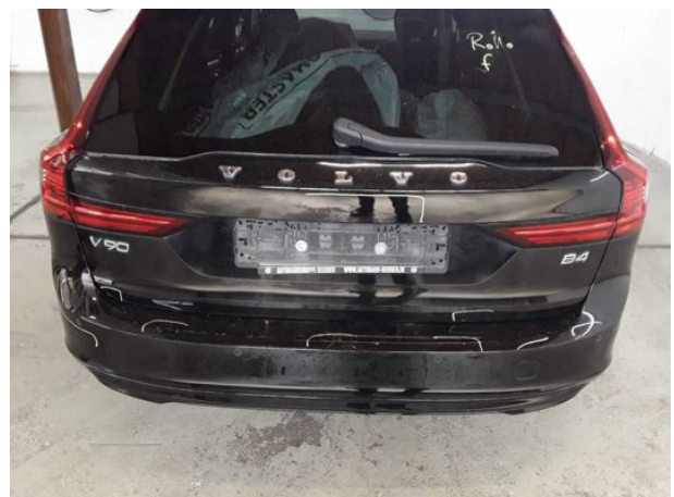
Damage #22: Boot lid / rear door: Boot lid - Scratched - Repair and paint
