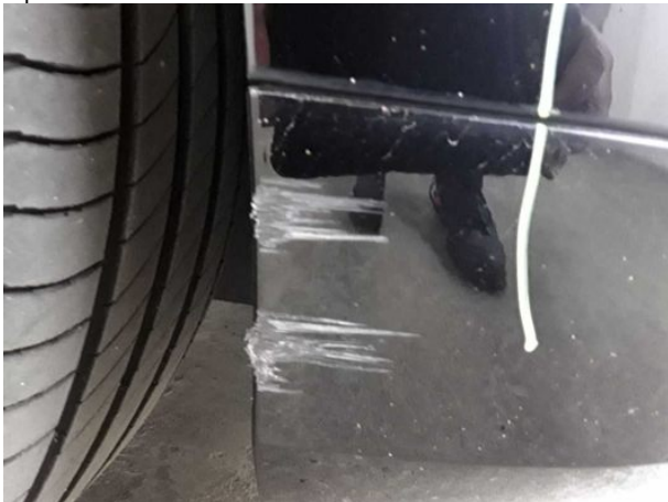
Damage #13: Front bumper: Spoiler - Scratched - Replace
