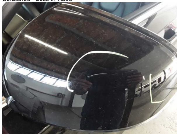
Damage #10: Wing mirror - left side: Cap - Scratched - Smart repair
