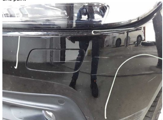
Damage #18: Rear bumper: Rear bumper - Scratched - Repair and paint
