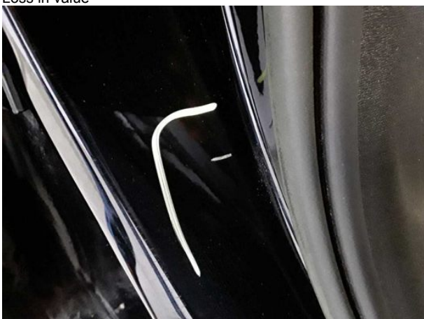
Damage #8: Sill - right side: Sill - Scratched - Smart repair
