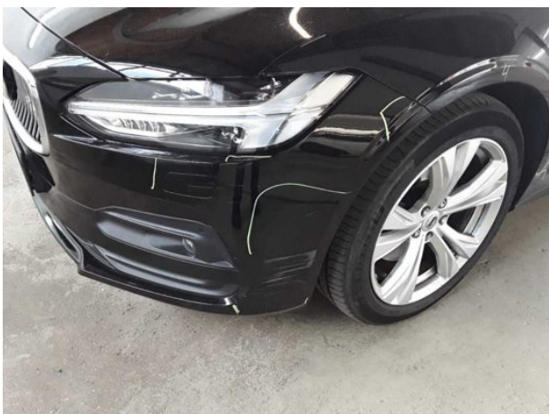
Damage #13: Front bumper: Spoiler - Scratched - Replace
