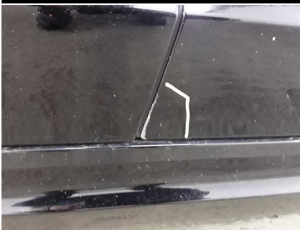
Damage #11: Door - front right side: Door - Scratched - Smart repair
