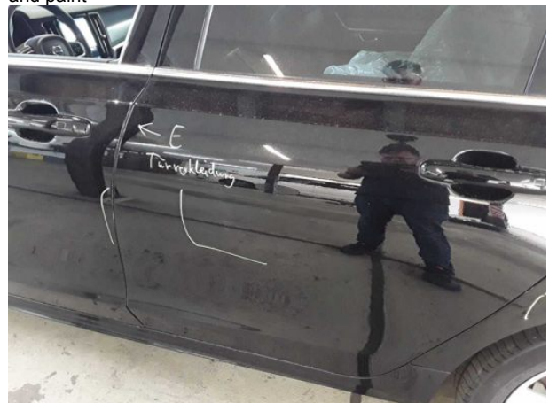
Damage #20: Door - rear left side: Door - Scratched - Paint
