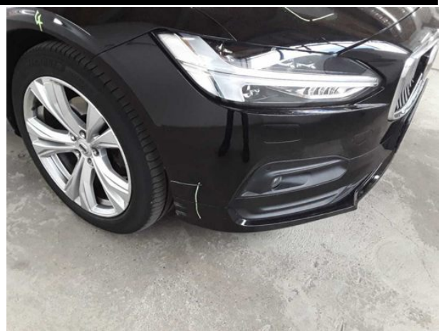
Damage #13: Front bumper: Spoiler - Scratched - Replace
