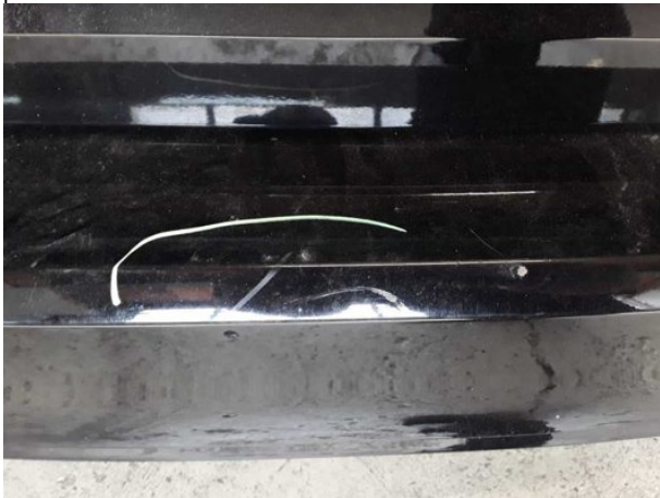
Damage #19: Rear bumper: Rear bumper - Scratched - Repair and paint
