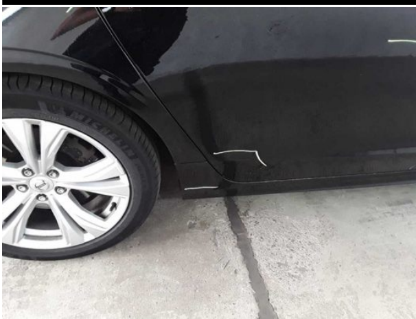
Damage #14: Sill - right side: Trim - Scratched - Paint
