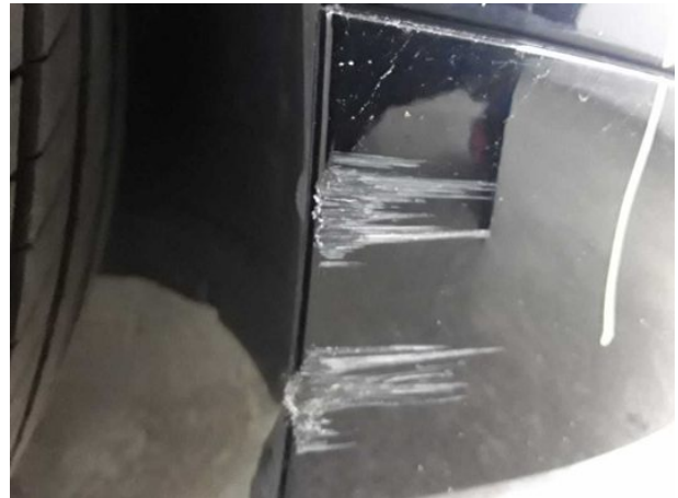
Damage #13: Front bumper: Spoiler - Scratched - Replace
