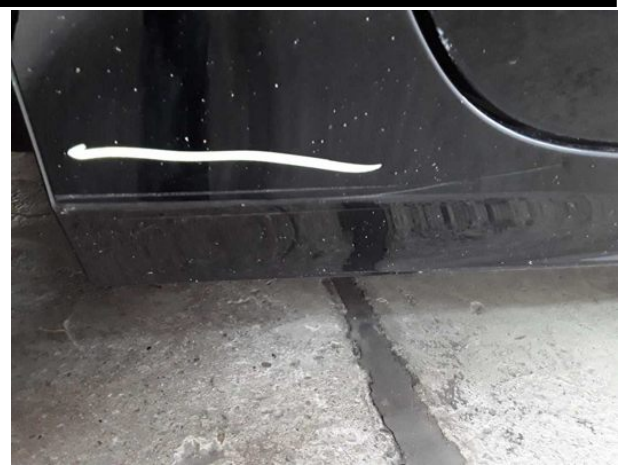
Damage #14: Sill - right side: Trim - Scratched - Paint
