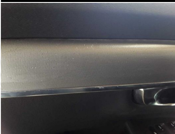
Damage #17: Trim / covers: Door trim - front left side - Scratched - Replace
