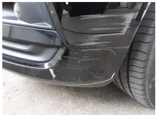
Damage #13: Front bumper: Spoiler - Scratched - Replace
