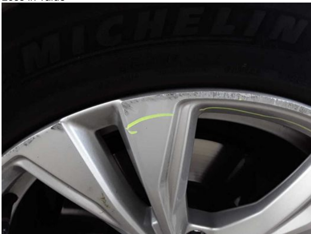
Damage #7: Wheel / tyres: Alloy rim - front right side - Scratched - Loss in value
