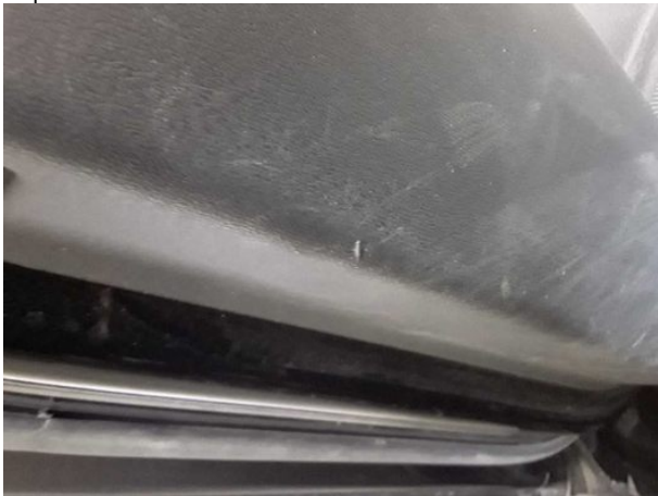
Damage #17: Trim / covers: Door trim - front left side - Scratched - Replace
