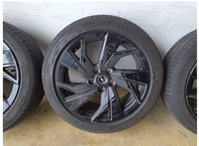
Damage 3: 2nd wheel set: 1 alloy rim - Scratch(es) - Smart repair
