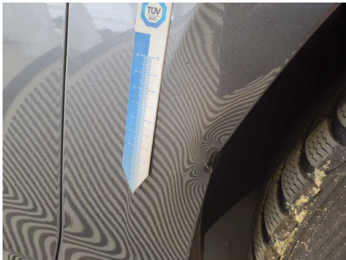
Damage 10: Mudguard - right side: Mudguard - right side - Deformed - Replace
