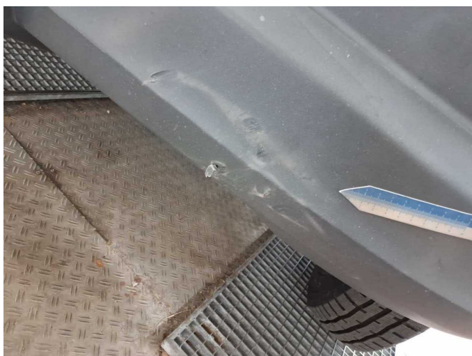
Damage 6: Front bumper: Front bumper - Damaged - Replace
