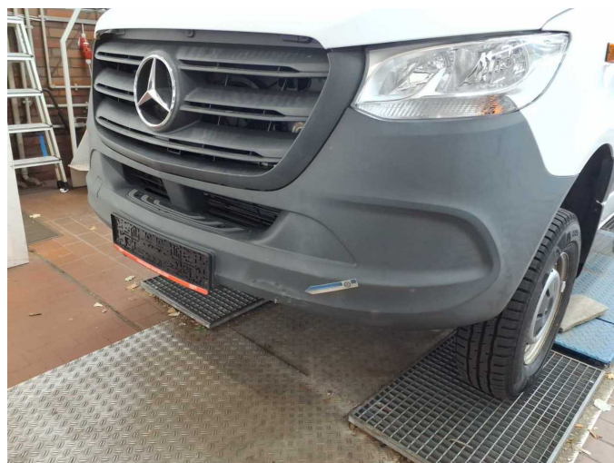
Damage 6: Front bumper: Front bumper - Damaged - Replace
