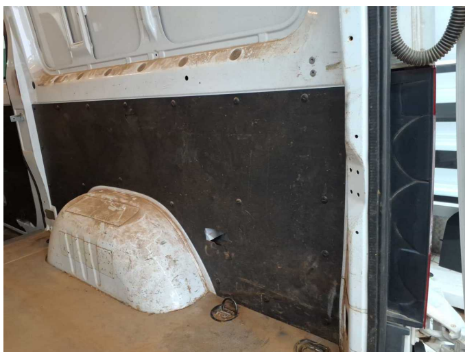
Damage 4: Side panel - rear right side: Interior trim - Broken / torn - Replace
