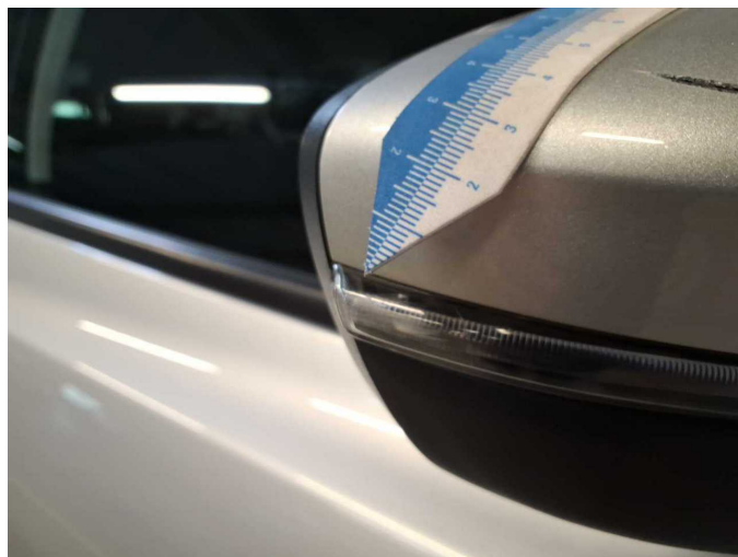
Damage 11: Indicator - front: Mirror - right side (Materialabtrag) - Scratched - Replace
