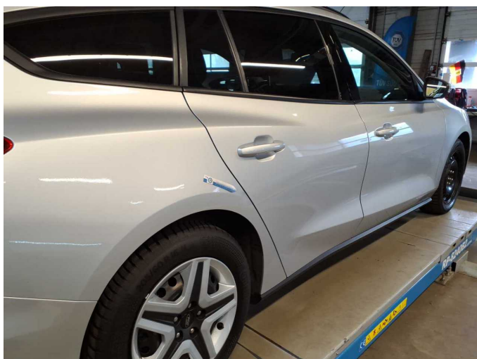
Damage 9: Side panel - rear right side: Side panel - dent(s) - Smooth repair work
