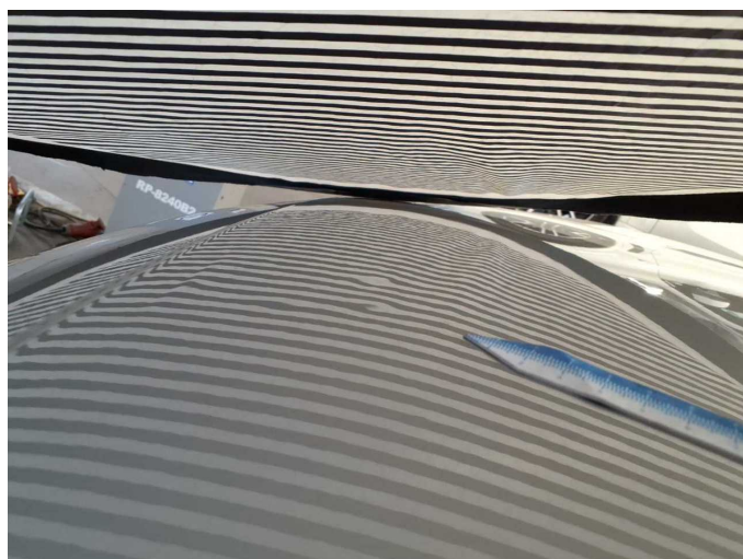
Damage 17: Bonnet: Bonnet - Deformed - Repair and paint
