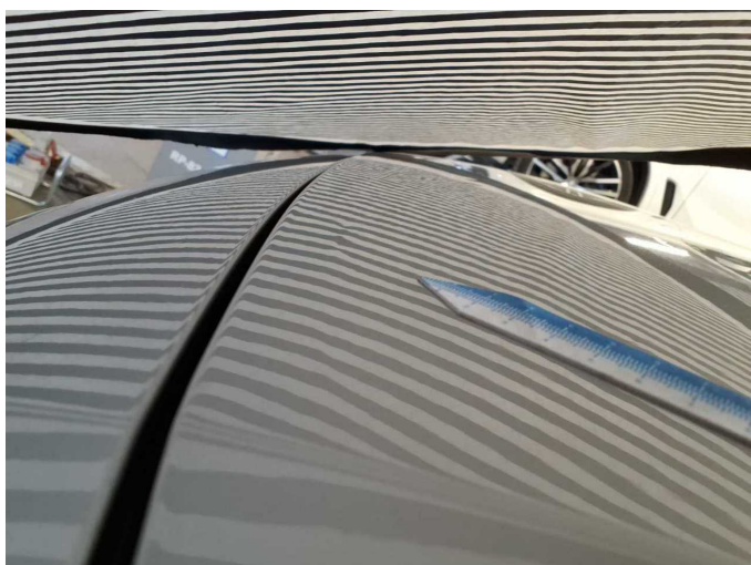
Damage 17: Bonnet: Bonnet - Deformed - Repair and paint
