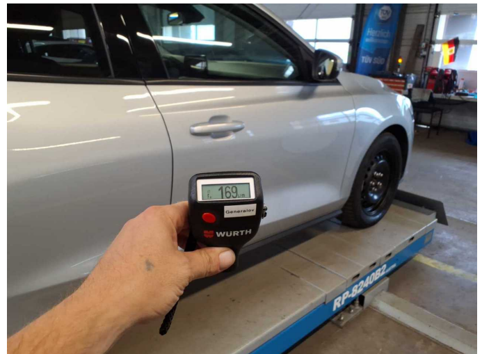
Repainting 2: Door - front right side
