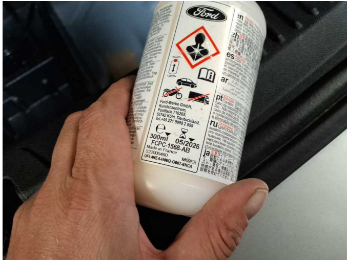
Damage 4: Equipment: Tirefit filler - Expired - Replace
