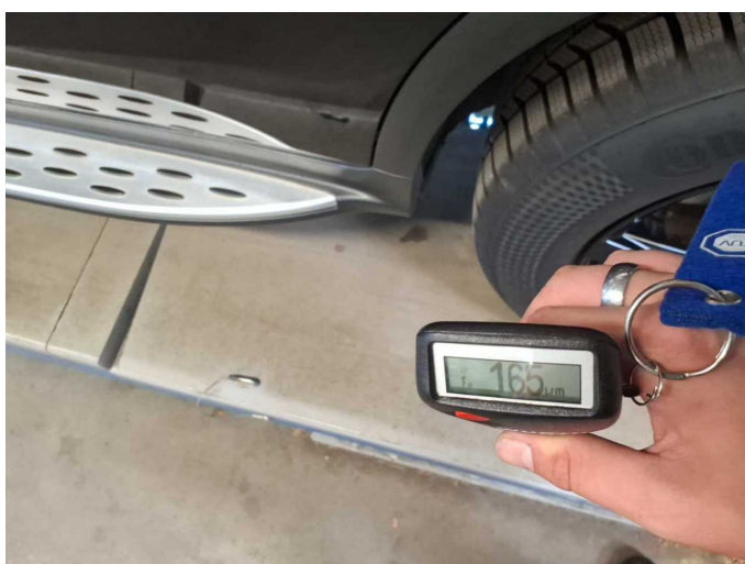
Side panel - rear left side: 165 µm
