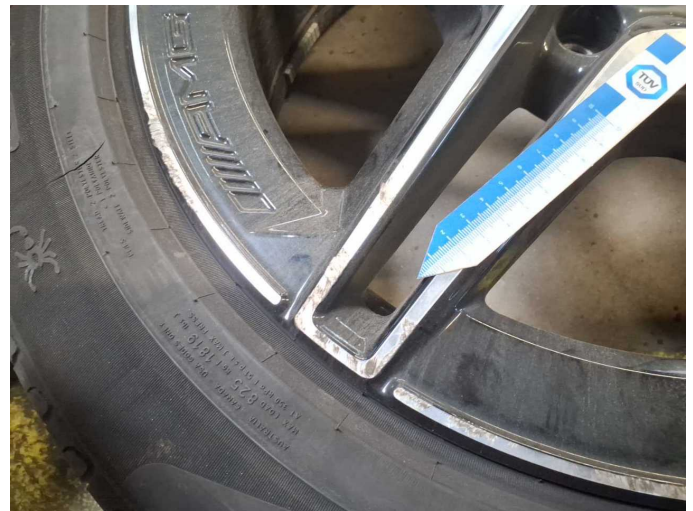
Damage 9: 2nd wheel set: 1 alloy rim - Scratched - Replace
