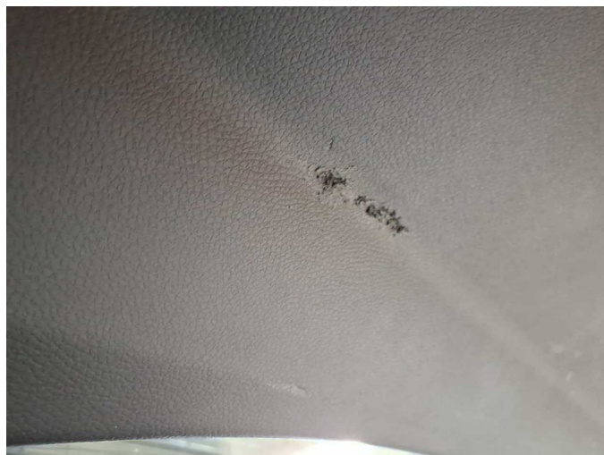
Damage 1: Trim / covers: Boot lid - interior trim - Scratched - Smart repair
