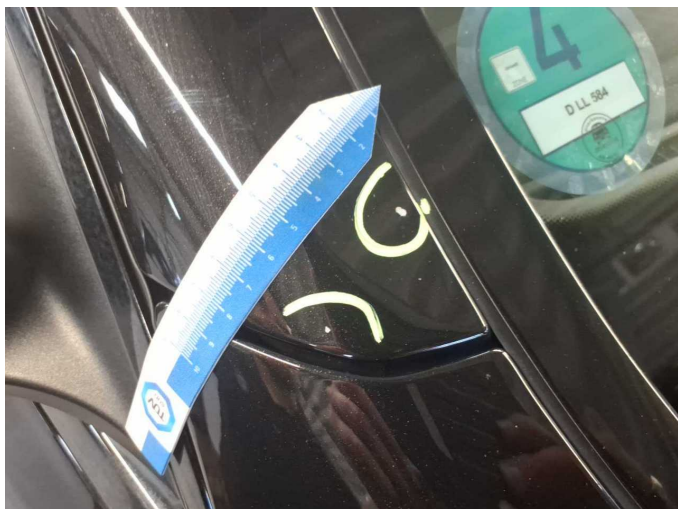
Damage 3: Body: A-pillar - right side - Stone chips - Smart repair
