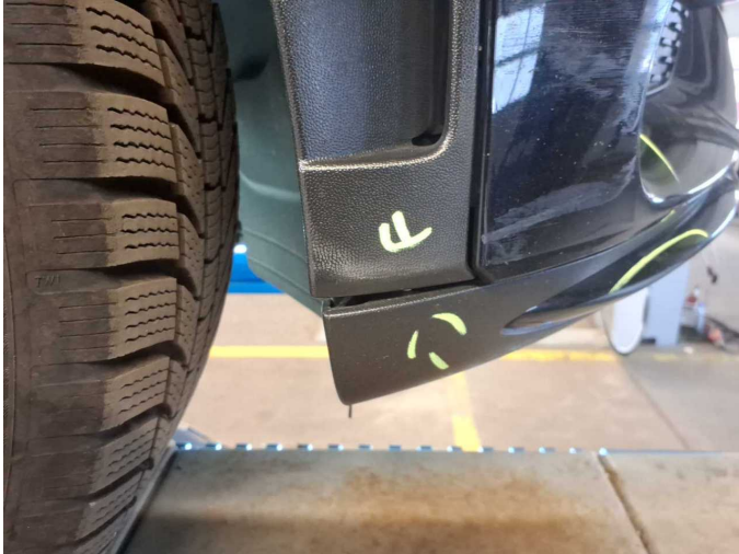
Damage 10: Front bumper: Front bumper (+ Blende+Leiste erneuern) - Scratched - Paint
