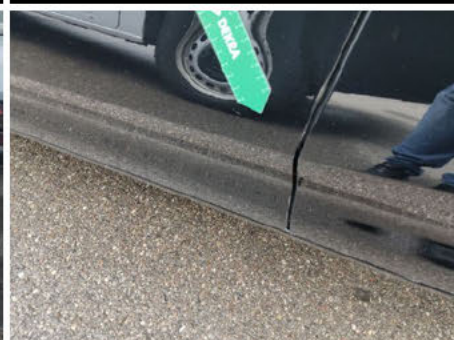
Tür / Vorne Links / Kratzer
