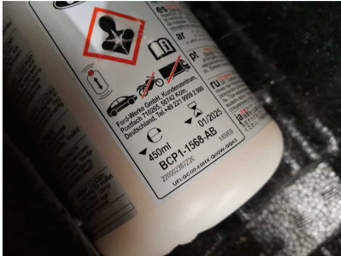
Damage 1: Equipment: Tirefit filler - Expired - Replace
