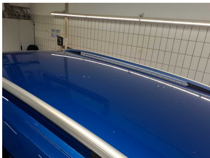
Damage 7: Roof: Roof - dent(s) - Smooth repair work
