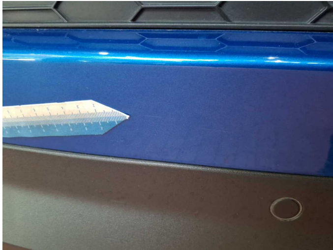
Damage 8: Rear bumper: Rear bumper - Scratch(es) - Paint
