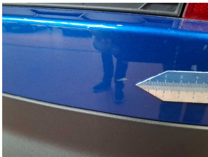
Damage 8: Rear bumper: Rear bumper - Scratch(es) - Paint
