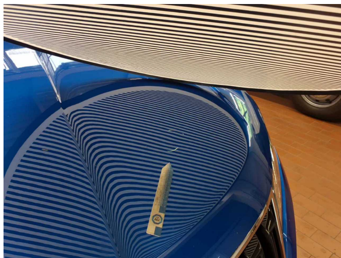
Damage 6: Bonnet: Bonnet - dent(s) - Smart repair
