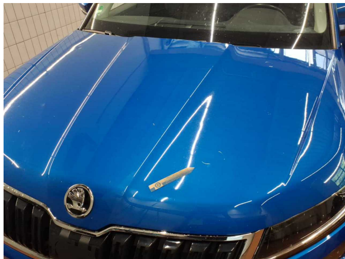
Damage 6: Bonnet: Bonnet - dent(s) - Smart repair
