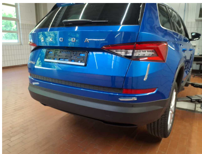
Damage 8: Rear bumper: Rear bumper - Scratch(es) - Paint
