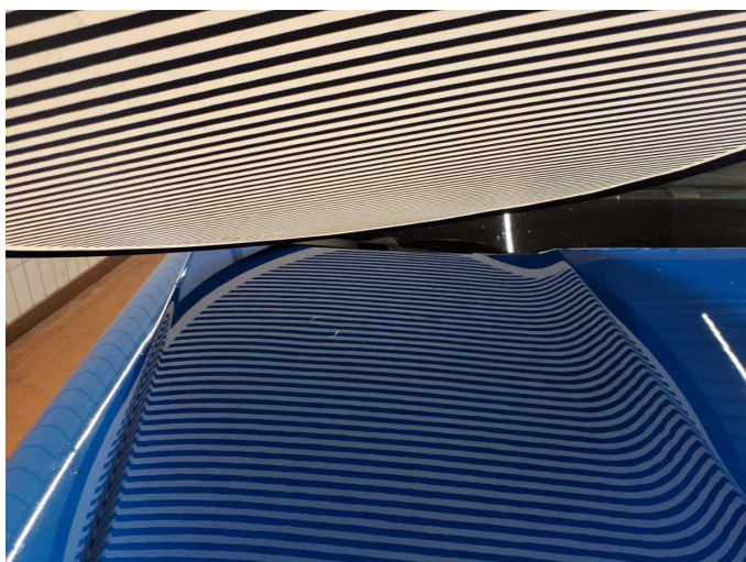
Damage 6: Bonnet: Bonnet - dent(s) - Smart repair
