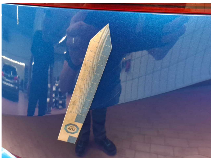
Damage 8: Rear bumper: Rear bumper - Scratch(es) - Paint
