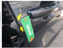
Roof pillar R, Scratch(es), Paint
