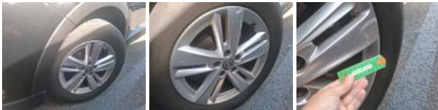
Tyre FL, Out of tolerance, Replace
