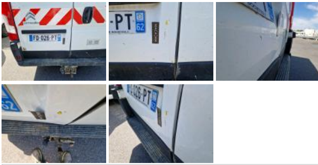
Rear light L, Broken, Replace
