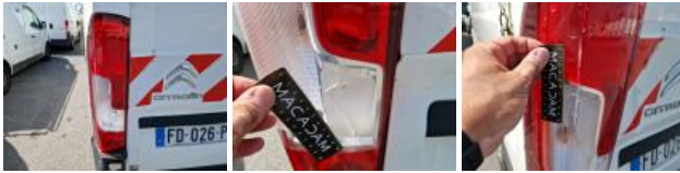
Rear light R, Broken, Replace
