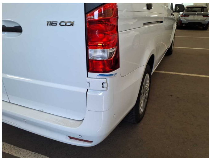
Damage 3: Rear bumper: Cover - bumper - rear - Scratch(es) - Smart repair
