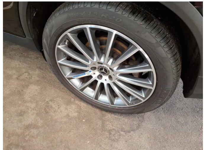
Damage 8: Wheel / tyres: Alloy rim - rear left side - Scratch(es) - Loss in value
