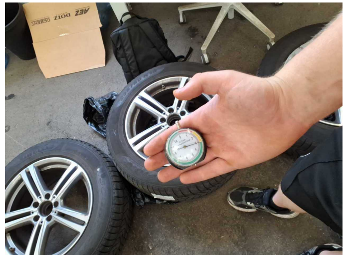
Damage 3: 2nd wheel set: 1 tyre - Does not meet the leasing specifications - Replace
