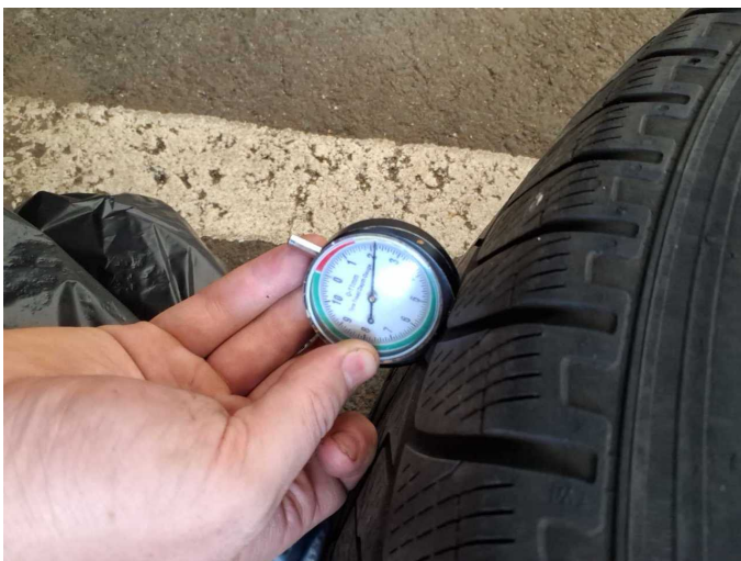
Damage 4: 2nd wheel set: 1 tyre - Worn - Replace
