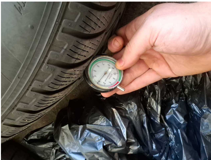
Damage 6: 2nd wheel set: 1 tyre - Does not meet the leasing specifications - Replace
