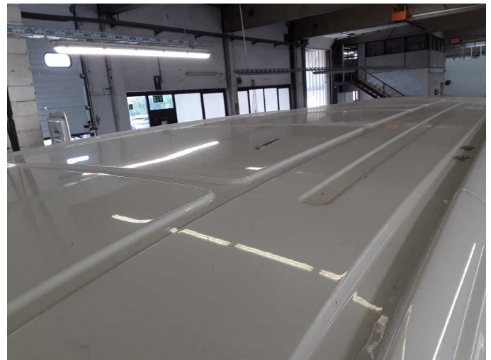
Damage 3: Roof: Roof - dent(s) - Smooth repair work
