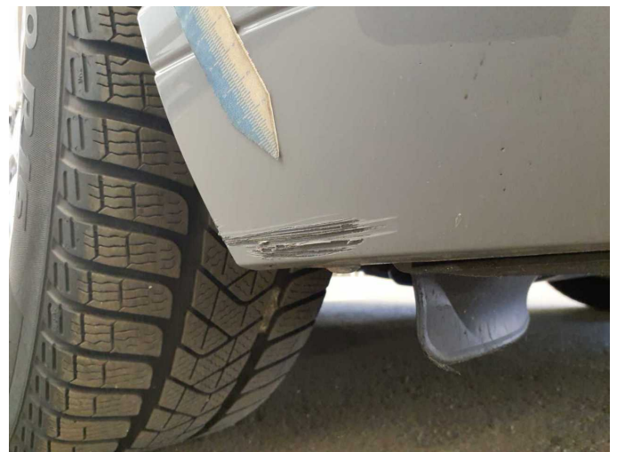
Damage 2: Front bumper: Front bumper - Scratch(es) - Paint
