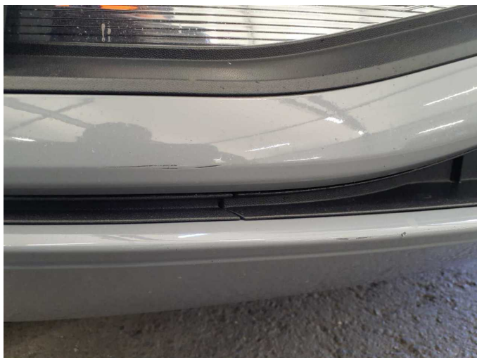
Damage 2: Front bumper: Front bumper - Scratch(es) - Paint
