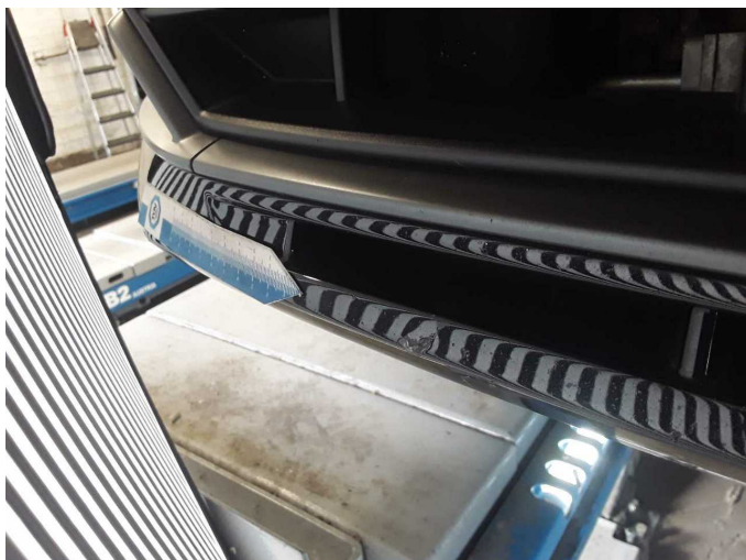
Damage 2: Front bumper: Front bumper - Dent / paintcoat damage - Smart repair
