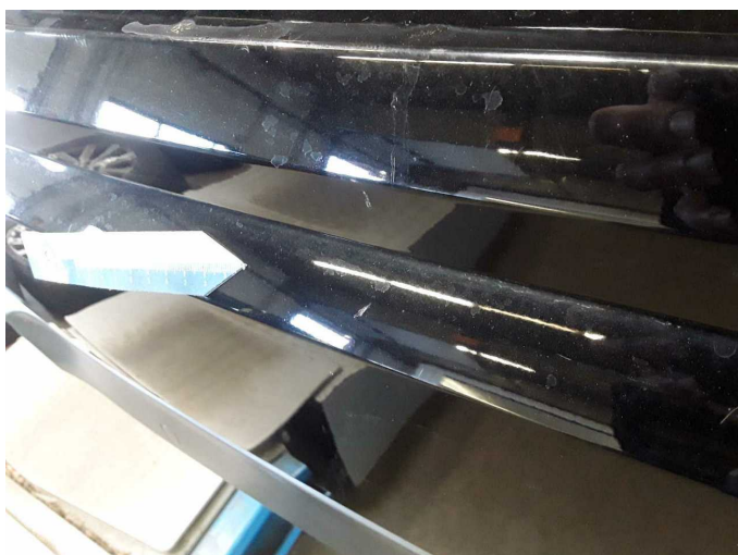
Damage 3: Rear bumper: Rear bumper - Scratch(es) - Paint
