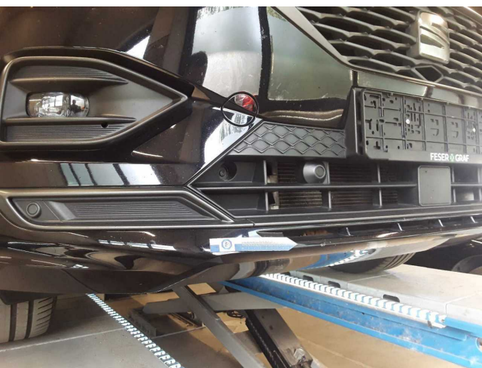
Damage 2: Front bumper: Front bumper - Dent / paintcoat damage - Smart repair
