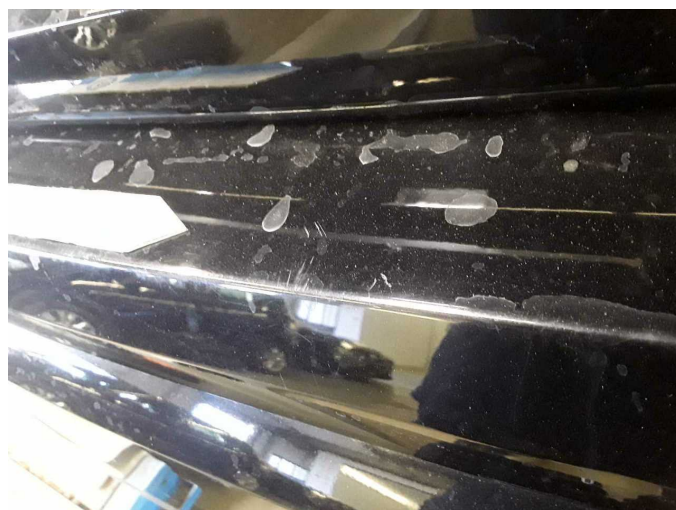
Damage 3: Rear bumper: Rear bumper - Scratch(es) - Paint
