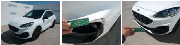
Bumper moulding FL, Scratch(es), Repair and paint (complete)
