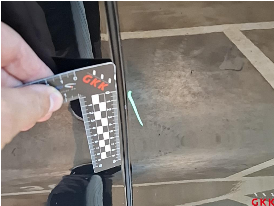
Picture 25 door front right, edge, scratched, disassemble, grind, polish
