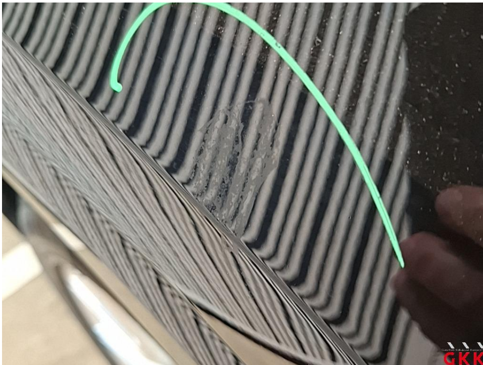
Picture 24 fender front right, paintwork eroded, prepare
