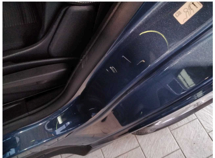
Damage 8: Body: C-pillar - left side - Dent / paintcoat damage - Smart repair
