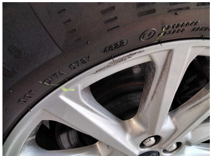
Damage 9: Wheel / tyres: Alloy rim - rear left side - Scratch(es) - Smart repair
