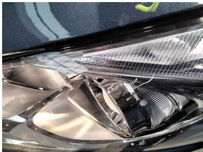
Damage 10: Headlight: Headlight - left side - Scratch(es) - Loss in value
