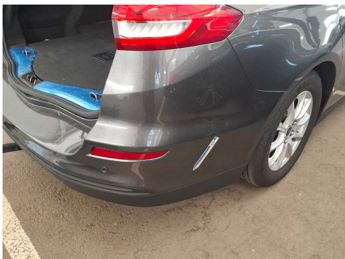
Damage 5: Rear bumper: Rear bumper - Scratch(es) - Paint
