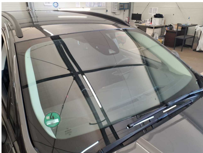
Damage 7: Vehicle glazing: Windscreen - Stone chips - Replace
