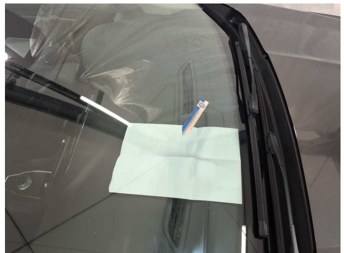
Damage 7: Vehicle glazing: Windscreen - Stone chips - Replace
