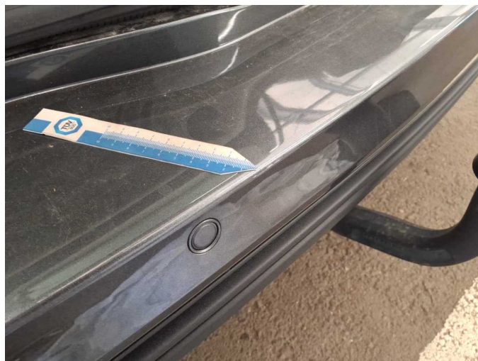
Damage 5: Rear bumper: Rear bumper - Scratch(es) - Paint
