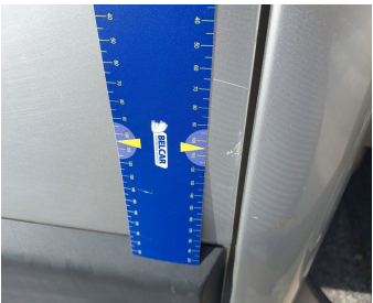
Door Rear Left // Repair & Painting-scratch + dent
