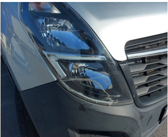
Light / Front Right / Replace-cracked
