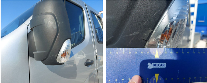
Side View Mirror Left / Direction Indicator / Replace-scratch
