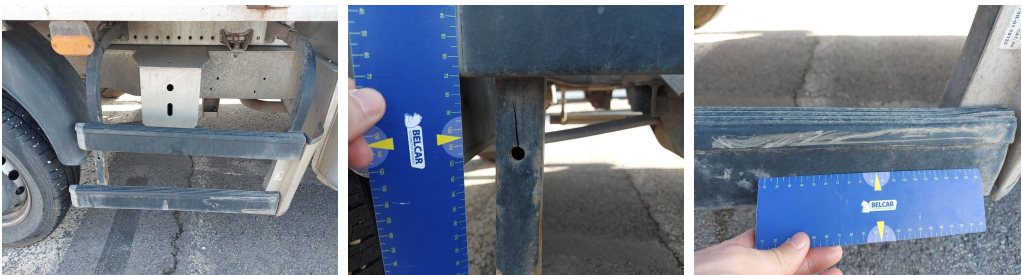
Rocker Panel Right / Cover Not Painted / Replace-Chipped paint
