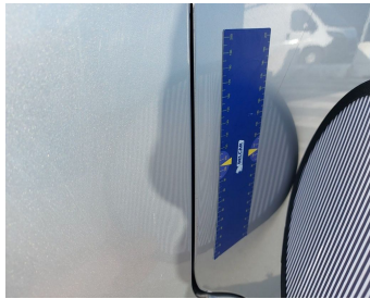
Door Front Left // Smart Repair Medium-dent
