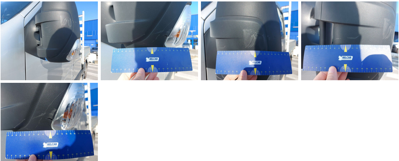
Side View Mirror Left / Shell / Replace Not Painted-cracked
