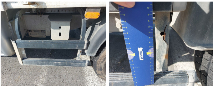
Rocker Panel Left / Cover Not Painted / Replace-Chipped paint
