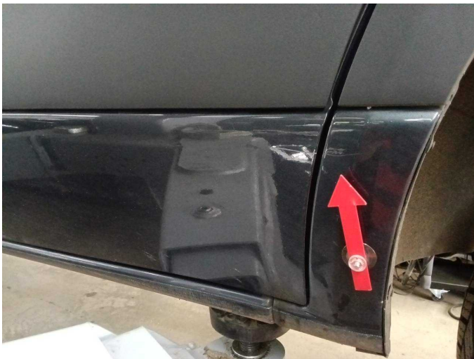
Damage 2: Sill - right side: Trim - Scratch(es) - Smart repair
