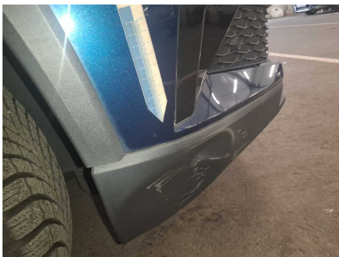
Damage 4: Front bumper: Front bumper (+Radlauf, + Spoiler) - Damaged - repair according to calculation
