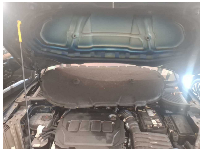
Damage 1: Bonnet: Insulation lining - Malposition - Un- / install
