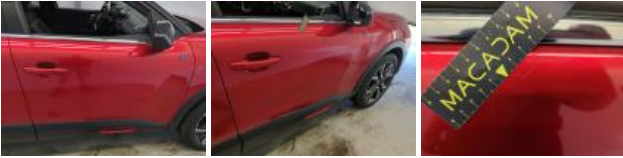
Door RR, Scratch(es), Repair and paint (complete)
