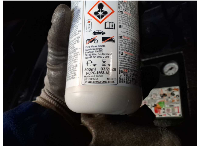
Damage 4: Equipment: Tirefit filler - Expired - Replace
