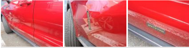
Step L, Dent(s) and scratch(es), Acceptable
