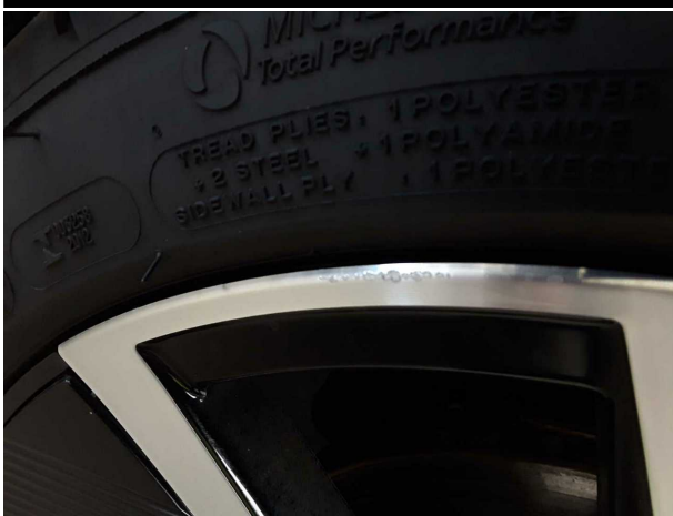
Damage #4: Wheel / tyres: Alloy rim - front right side - Scratched - Loss in value
