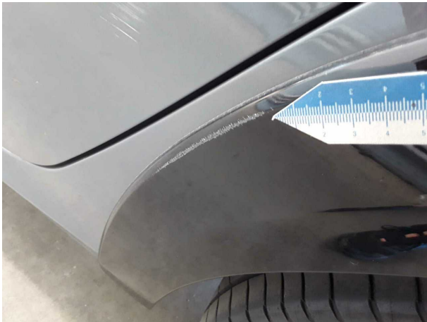
Damage #5: Side panel - rear left side: Wheel well extension - Scratched - Paint
