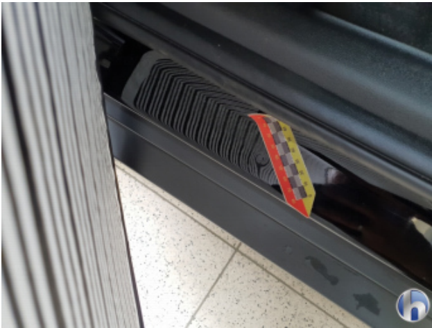
2. Türeinstieg Vorne - Links 1 Delle - Smart Repair
