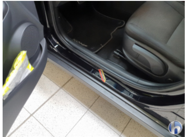
2. Türeinstieg Vorne - Links 1 Delle - Smart Repair
