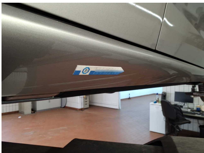
Damage 4: Sill - right side: Trim - Scratched - Paint
