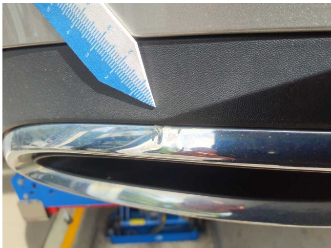
Damage 3: Rear bumper: Rear bumper (Blende) - Paint defect - Replace
